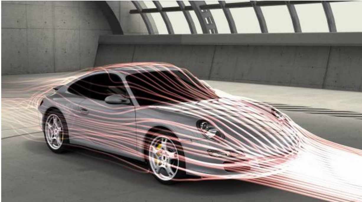
RTT RealFluid: physically accurate airflows are displayed on a model in real time.
