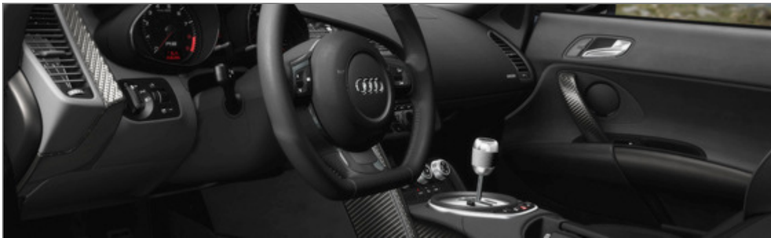
Photo-realistic visualization of the Audi R8 interior created using RTT RealLight – shadowing effects are computed using "Ambient Occlusion" functionality.
